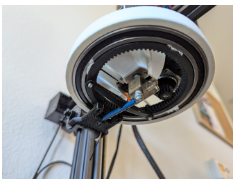
Fig. 3. Bottom-up view of the printer showing the rotational axis gearing, spool holder, and guide tube.
