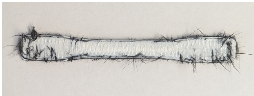
Fig. 6. Printed sample specimen with carbon fiber.
